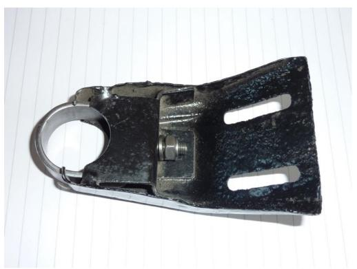
This inner clamp was then assembled into the 'underdash' outer bracket, ready to be fitted over the steering column, tightened-up and secured to the underside of the dashboard.
