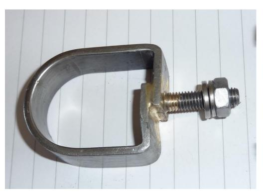
for the threaded stud. Finally, bronze 'welding' it all together and fitting a nut and locking washer as shown in the photo.
